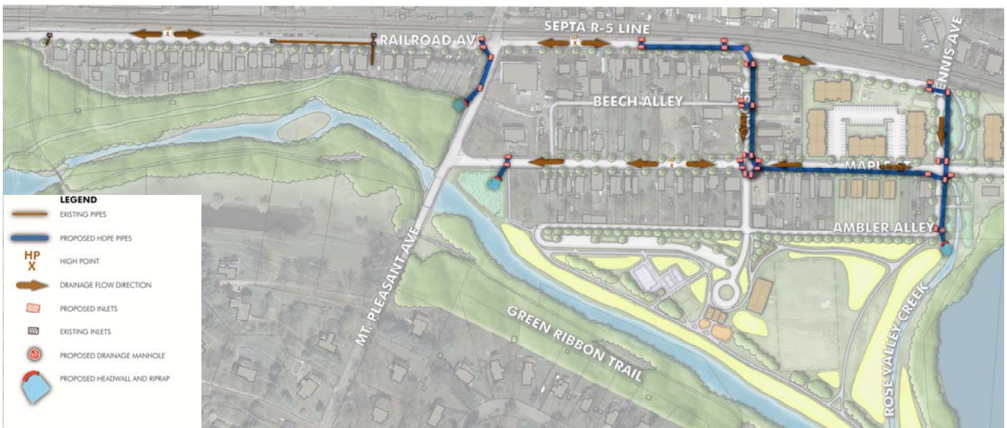
Figure 2.5 Conceptual Storm Sewer Plan
