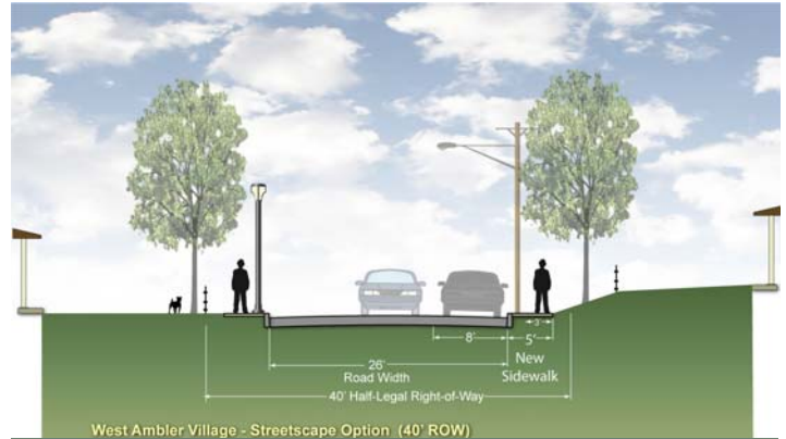
Figure 2.6 Typical streetscape improvement section.
